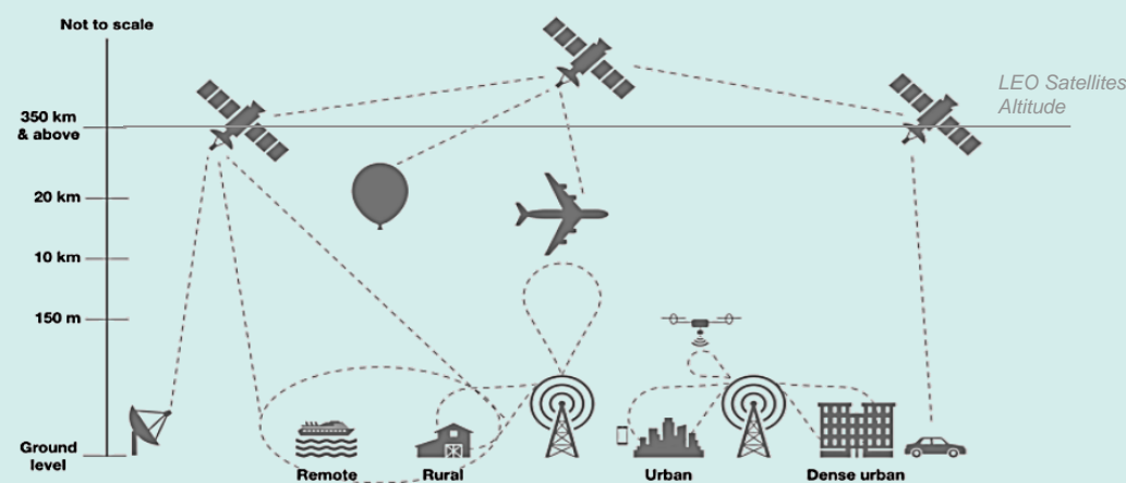
FIGURE 9: 6G coverage provided by integrating terrestrial networks with LEO satellite access
